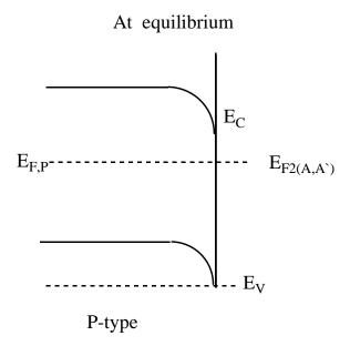
Fig.(1): Band diagram and charge – carrier profiles of n – type and  $\,p\,$ -type semiconductor / liquid junctions.  $E_c$ ,  $E_v$ , are conduction and vavenee band energy,  $E_F$  is the Fermi energy,  $e^{\cdot}$ , and  $\,h^{^+}$  are electron and hole respectivity [5].
