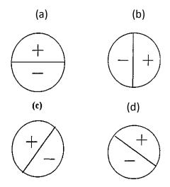
These masks are use to detect edges in four directions, a) horizontally, b) vertically, c) from top right to left down, and d) from top left to right down
