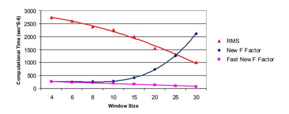
Fig. (2) The total computational time to find the match window for the three methods
