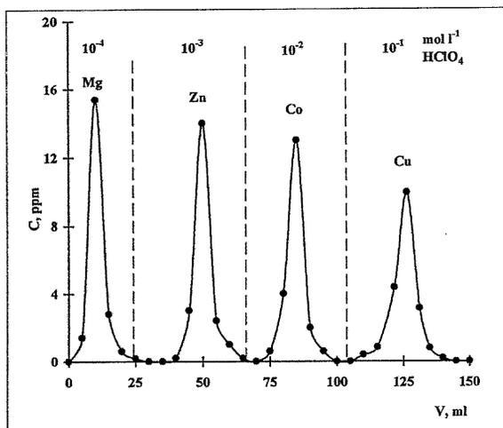
Fig.6 Separation of metal ion mixtures containing 100  $\mu\text{g}$  of each metal ion, on LiChroprep RP-8 treated with a mixture of Aliquat 336 and Titan Yellow. Column packed with 5 g of sorbent. Mean flow rate:  $1\text{ ml min}^{-1}$
