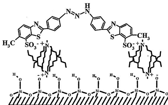
Fig.3 Silica impregnated with Aliquat 336 and modified with ion pairs composed of cation of Aliquat 336 and anion of Titan Yellow
