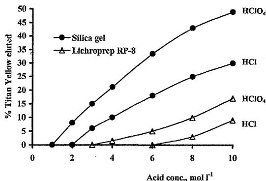
Fig.5 Percent of Titan Yellow eluted from silica and LiChrorep RP-8 modified with a mixture of Aliquat 336 and Titan Yellow as a function of concentration of  $\text{HClO}_4$  and  $\text{HCl}$  acids used as eluents
