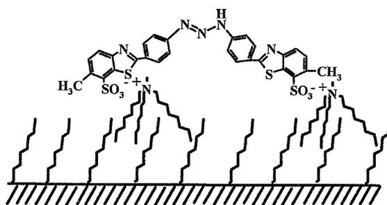
Fig.4 LiChrorep RP-8 modified with ion pairs composed of cation of Aliquat 336 and anion of Titan Yellow
