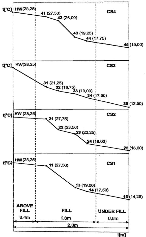
Fig. 5 Vertical water temperature distribution according to Table 2
