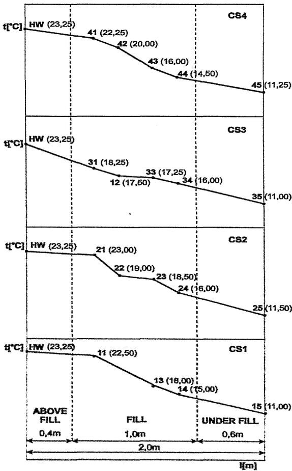
Fig. 4 Vertical water temperature distribution according to Table 1
