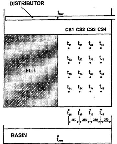
Fig.2 Thermoelements arrangement in the investigated cooling tower
