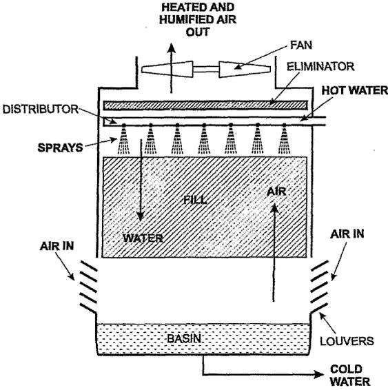
Fig.1 Wet counterflow cooling tower
