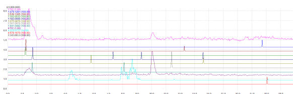
Figure 2: HPLC-ESI-MS analysis of the nettle extract (5 min extraction) with the addition of 0.1% formic acid to the mobile phases. TIC in the positive mode – Top: TIC in the negative mode – Bottom and Middle: EIC records of identified phenolic compounds included.
