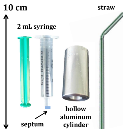
Figure 1: The photo of the components used to build a miniature EBC sampling device.
