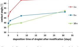
*Figure 1:* Dependence of the contact angle of droplets of 0.5 mM trisodium citrate solution on the PET surface modified by DCSBD after one, five and ten seconds; droplets were deposited immediately as well as one, seven and 31 days after the modification.
