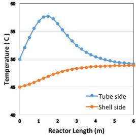
*Figure 4.* Temperature profiles of the reactor and coolant.
