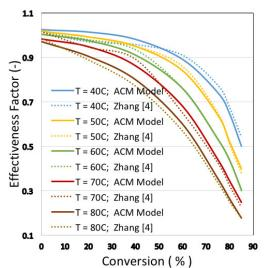
*Figure 2.* Effectiveness factor for the MTBE synthesis reaction based on data from Ref. [4].
