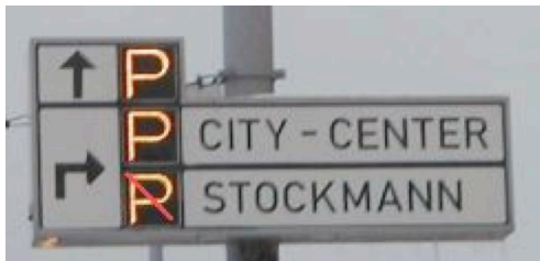
Figure 5. Variable message signs for parking as part of the HelUTC system.
