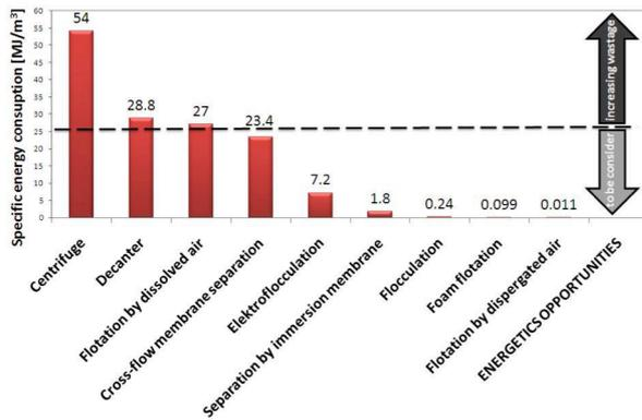
Figure 4: The energetic consideration of selected separation processes (the dashed line shows the energy content of algae suspensions on average of  $25 \text{ MJ m}^{-3}$ )
