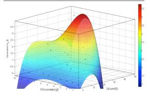
Figure 4: Generated H<sub>2</sub> as a function of KOH concentration and dry cell current
