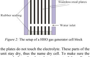
unit stay dry, thus the name dry cell. To make sure the gas made from the electrolyte gets out of the cell and the solution flows between the plates, there are holes on the top (for the gas) and bottom (for the electrolyte) on the metal slats (*Fig.1*).
