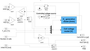
*Figure 5:* Matlab Simulink model of the HHO cell. The functional blocks implementing *Eqs.(5)* and *(6)* are denoted by different background colours
