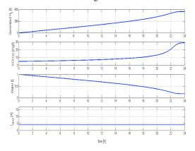
*Figure 6:* Simulation of a cell model with a constant current of 5 A for 1 day
