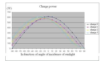
*Figure 5:* Charging power in function with the angles of the light
