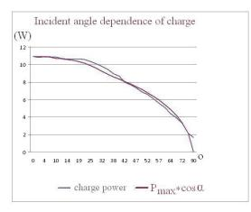
*Figure 4:* The measured and calculated performance of a cell
