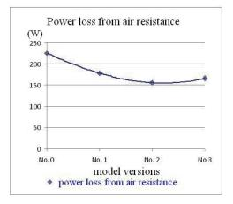
*Figure 3:* The change in the drag power of each model at 8 m/s
