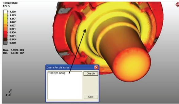
Figure 3: Surface temperature is 1133 °C at a properly measurable location
