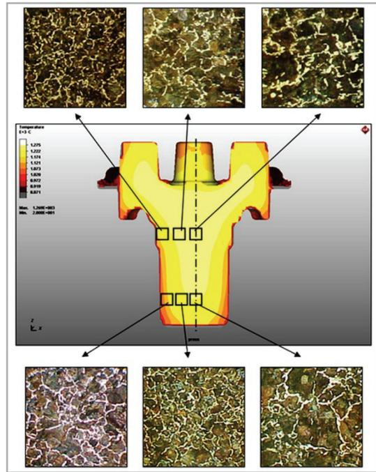
Figure 9: Relationship between the internal heat distribution and the microstructure
