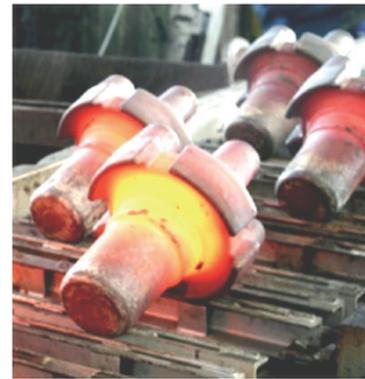
Figure 5: Planetary carriers cooled in cooling equipment, in air flow
