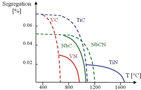
Figure 1: Example for segregation of micro-alloys
