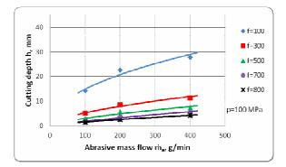
*Figure 6:* Effect of the abrasive mass flow rate on the depth of kerf at different feedrates and pressures, on AlMgSi0,5 aluminium alloy
