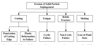
Figure 1: Material removal processes in course of solid particle erosion
