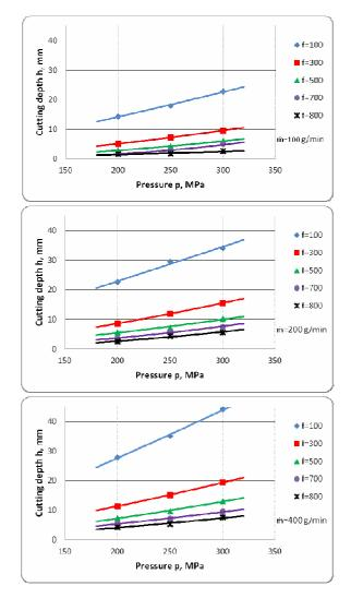
*Figure 5:* Effect of the pressure on the depth of kerf at different feedrates and abrasive mass flow rates, on AlMgSi0,5 aluminium alloy
