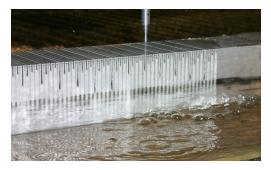
Figure 3: Kerfing tests in AlMgSi0,5 Aluminium Alloy
