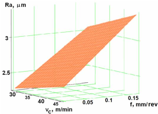
Figure 7: The changes of the average surface roughness in cutting speed and feed rate depending on dry machining with sharp tool
