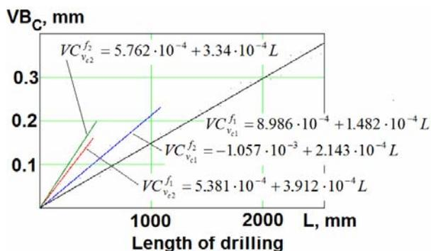
Figure 11: The changes of the corner wear in cutting speed and feed rate depending on dry machining
