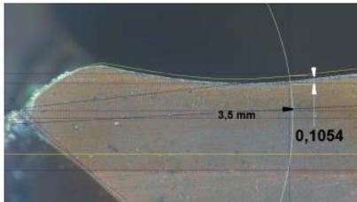
Figure 4: The worn drill L=1350 mm (M=300)
