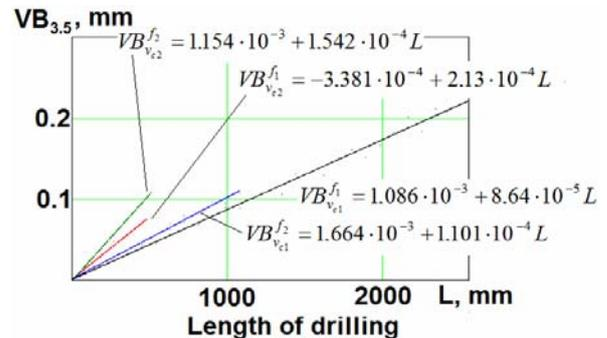
Figure 10: The changes of the flank wear in cutting speed and feed rate depending on dry machining
