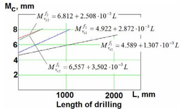
Figure 9: The changes of the torque in cutting speed and feed rate depending on dry machining
