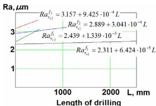
Figure 12: The changes of the average surface roughness in cutting speed and feed rate depending on dry machining
