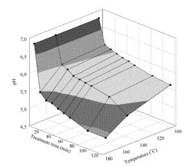
Figure 4: Acidity of grain sorghum stover slurries as the function of LHCW contact time and temperature (•: experimental data point)
