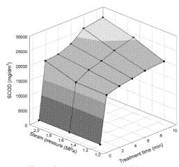
Figure 5: Effects of steam pressures on SCOD concentration levels of grain sorghum stover slurries as the function of the contact time during steam explosion (•: experimental data points)
