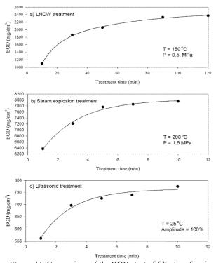
*Figure 11*: Comparison of the BOD<sub>5</sub> test of filtrates of grain sorghum stover slurries after various pre-treatment methods
