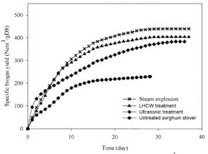
*Figure 12*: Specific cumulative biogas yield (Ncm<sup>3</sup>/g DS) of grain sorghum stover substrates after pre-treatments
