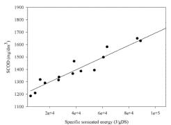
Figure 8: SCOD change in grain sorghum stover slurry as a function of specific sonication energy (●: experimental data points)
