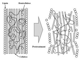
Figure 1: The disintegration of lignocellulosic material by pre-treatments
