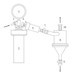
*Figure 2:* Scheme of the steam explosion apparatus (1. input valve, 2. steam generator, Parr 4843 reactor, 3. pressure gauge, 4. evacuation valve, 5. steam inlet valve, 6. digester vessel, 7. expansion valve, 8. cyclone, 9. sampling valve, 10. steam
