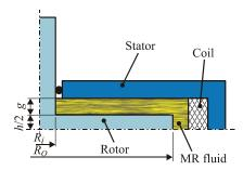
Figure 2: MR fluid disk brake simplified representation
