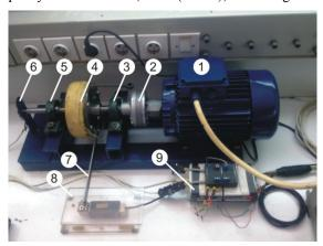
Figure 3: Demonstrating the test rig for MR brake 1. drive, 2. coupling, 3. self-aligning ball bearing, 4. MR fluid brake, 5. self-aligning ball bearing, 6. optical encoder, 7. load arm, 8. load cell, 9. data acquisition card
