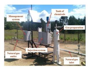
Figure 2: Chemical injection system on a gas well
