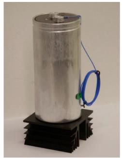
Figure 7: Core temperature measurement of a capacitor
