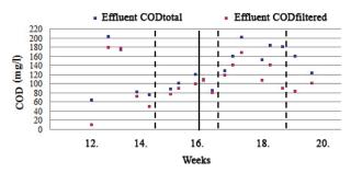
Figure 5: COD removal in the 50% CNT reactor
