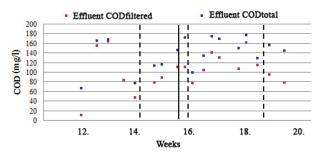
Figure 3: COD removal in the control reactor
