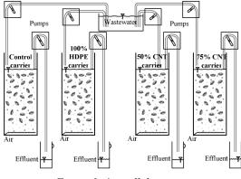
Figure 1: 4 parallel reactors
