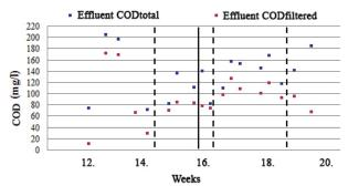
Figure 4: COD removal in the 100% HDPE reactor
