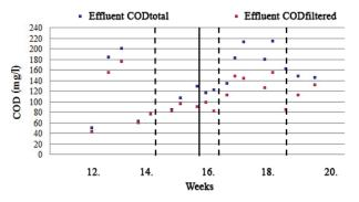
Figure 6: COD removal in the 75% CNT reactor
