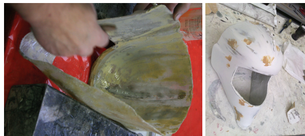
Figure 6: Separating the prototype form and filling the prototype model
