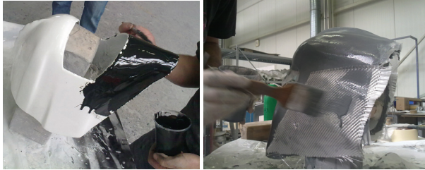
Figure 7: Brushing the gelcoat and laminating the production form
