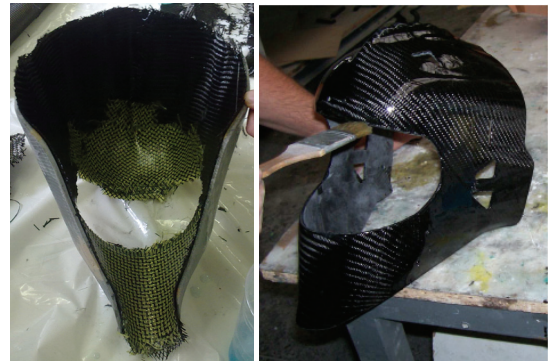
Figure 8: Reinforced chin and forehead with carbon-kevlar and the last layer of resin
