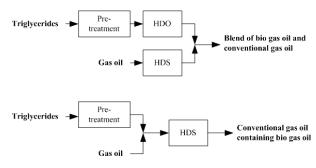
*Figure 3:* Options of the catalytic conversion of the vegetable oil-gas oil mixtures.
