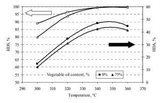
*Figure 9:* The changes in desulphurisation(HDS)- and dearomatization(HDA) efficiency as a function of temperature (p = 80 bar, LSHV = 1,0 h<sup>-1</sup>)
