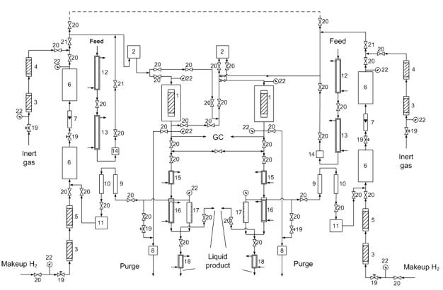
Figure 4: Simplified scheme of the test apparatus
