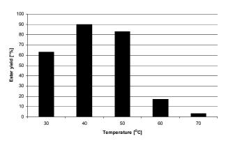
*Figure 3:* Effect of temperature on the relative value of esterification activity of immobilized lipase
