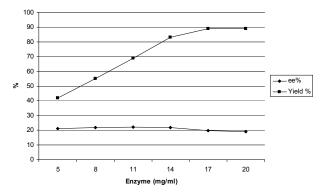
*Figure 4* : Effect of enzyme concentration on the enzymatic esterification of lactic acid by ethanol
