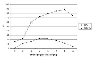
*Figure 2:* Effect of the molar ratio of alcohol to lactic acid on enantioselectivity of esterification of racemic lactic acid with ethanol, catalyzed by candida antartica
