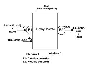
*Figure 7:* Schematic diagram of enantioselective transport of (L)-lactic acid through a lipase-facilitated SLM based on an ionic liquid
