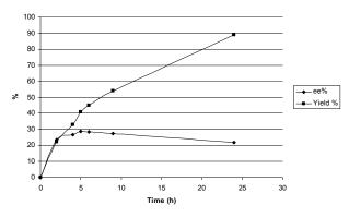
*Figure 6:* A time course of the esterification between lactic acid and ethanol by Novozymes 435
