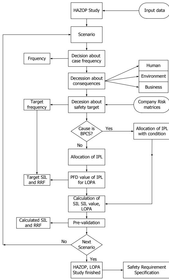
Figure 1: Method of SIL calculation
