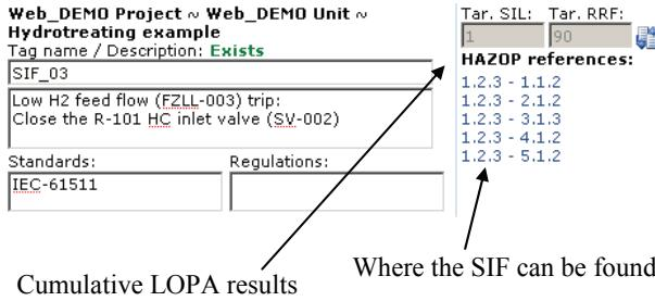
Figure 6: Example for result of a cumulative LOPA
