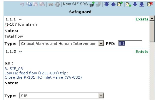
Figure 7: Edit safeguards in Tool4S SW
