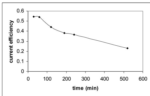
Figure 8: The change of current efficiency as a function of time
