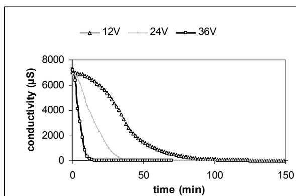
Figure 6/a: Conductivity of the diluate solution as a function of time
