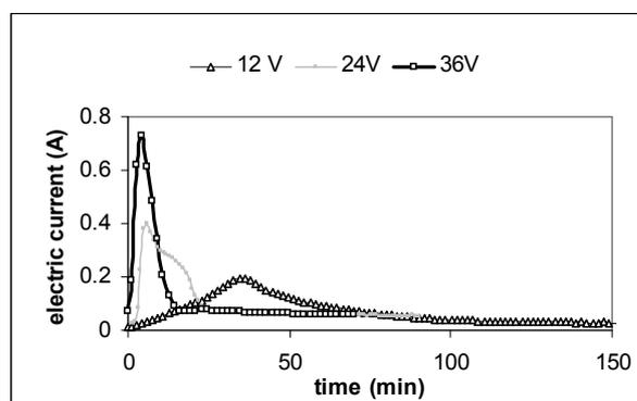
Figure 3: Electric current in the EDBM cell
