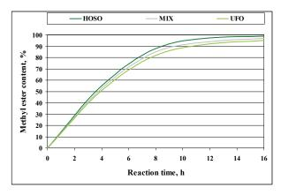
*Figure 1:* Methyl ester content of products as a function of transesterification time (catalyst Candida antarctica (Novozym 435))
