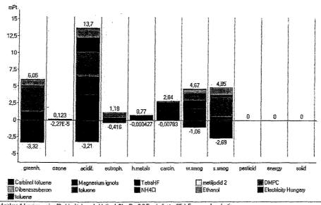
Analyse 1 kg processing 'Carbinol toluene'; Method: SimaPro 3.0 Eco-indicator 95 / Europe g / evaluation
