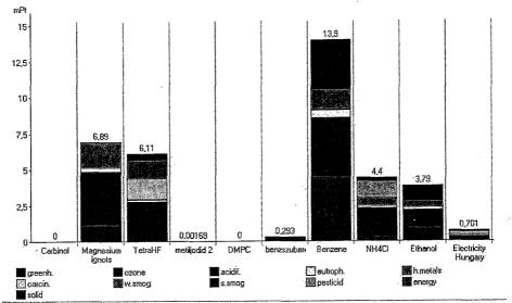
Analyse 1 kg processing 'Carbinol'; Method: SimaPro 3:0 Eco-indicator 95 / Europe g / indicator
