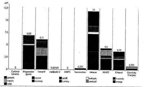
Analyse 1 kg processing 'Carbinol toluene'; Method: SimaPro 3.0 Eco-indicator 95 / Europe g / indicator
