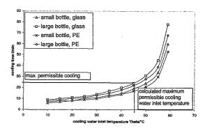
Fig.5 Result of calculation of cooling time
