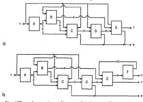
Fig.4 Flow sheet w/o cooling pond (a/b resp.) Flows: 1 Fresh Water; 2 Demineralised Water; 3 Recirculated Steam; 4
