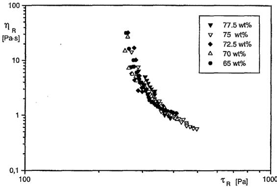
Fig.6 Reduced viscosity ( $\eta_R$ ) vs. reduced shear stress master curve for the alumina slips investigated.
