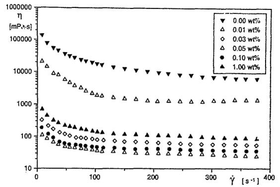
Fig.8 Apparent viscosity ( $\eta$ ) vs. shear rate ( $\dot{\gamma}$ ) flow curves for the 77.5 wt% alumina + sodium polyphosphate suspensions studied.
