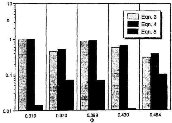
Fig.5  $n$  parameter values variation with solid volume fraction ( $\Phi$ ) for the alumina suspensions studied.
