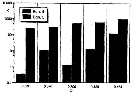
Fig.4 Consistency values ( $K$ ) variation with solid volume fraction ( $\Phi$ ) for the alumina suspensions studied.
