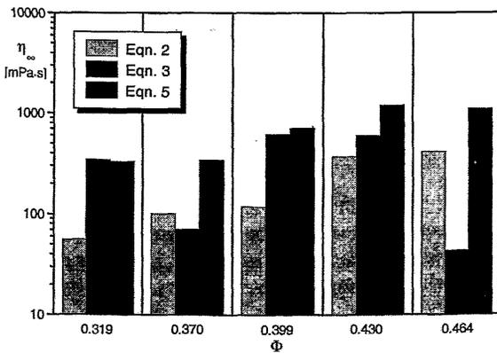
Fig.3 Infinite viscosity ( $\eta_\infty$ ) variation with solid volume fraction ( $\Phi$ ) for the alumina suspensions studied.
