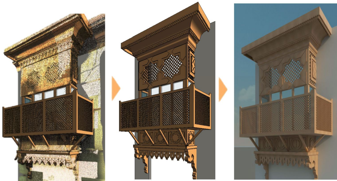
Figure 2: Creation and visualisation of a 3D model based on a point cloud [4]
