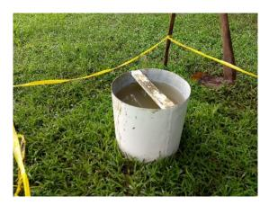
Figure 3. The soil infiltration measurement on the test plot
