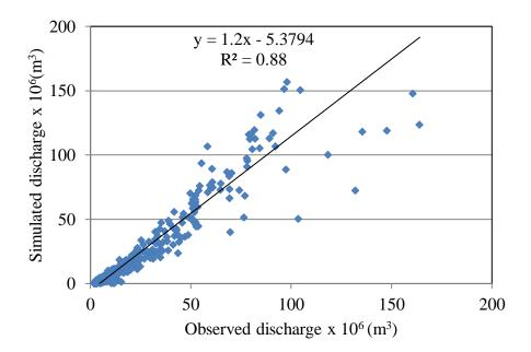
Figure 7. The WEAP model validation
