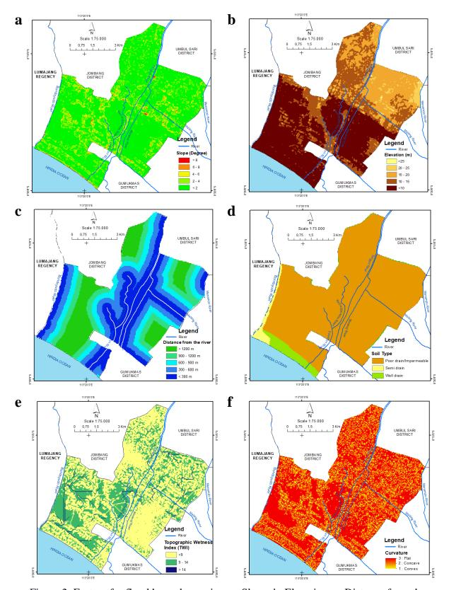
Figure 2. Factors for flood hazard mapping: a. Slope; b. Elevation; c. Distance from the river; d. Soil Type; e. Topographic Wetness Index (TWI); f. Curvature
