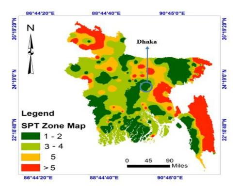
Figure 6. Zonation map using Standard Penetration Test (SPT)
