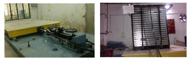
Figure 2. Shake table test apparatus Figure 3. Laminar box mounted on shake table A Laminar box was constructed on the shake table apparatus to reduce boundary effects wherever possible. The Laminar box neither resists nor promotes soil displacement to
