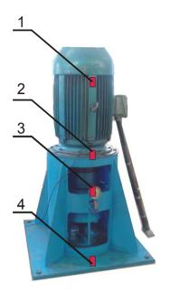
Fig. 5 Measuring points at well pump aggregate BP 350-3G, No. 1
