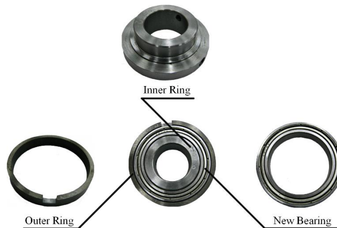
Fig. 3 Inner, outer rings and new bearing before and after assembly
