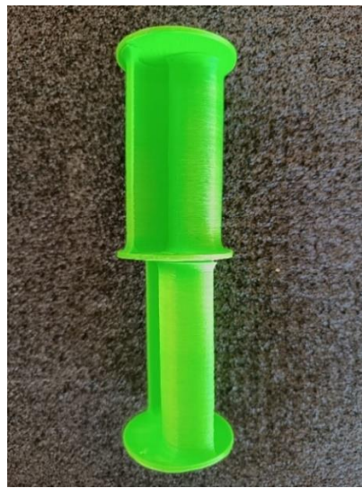
Fig. 8 Savonius turbine printed in 3D and assembled, developed by authors
