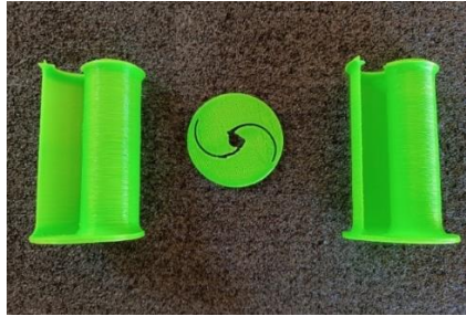
Fig. 7 Savonius turbine printed in 3D, developed by authors
