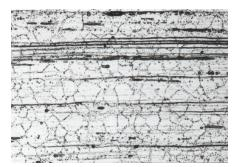
Figure 3a: "5" steel microstructure -Longitudinal section (x 200).
