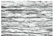
Figure 4a: "4L" steel microstructure -Longitudinal section (x 200).
