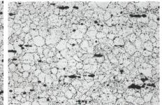
Figure 3c: "5" steel microstructure -Radial section (x 200).
