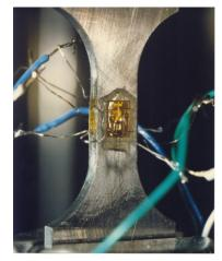
Figure 8: Specimen (B) during tensile test.
