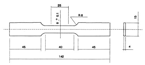
Figure 5: Standard specimen (S) for tensile test.
