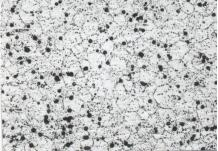
Figure 3b: "5" steel microstructure -Transversal section (x 200).
