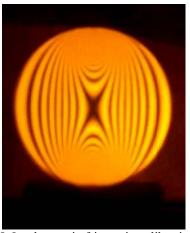
Figure 5. Isochromatic fringes in calibration disk.
