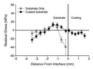
Figure 13: Residual stress measurement of CS Al coating [60].
