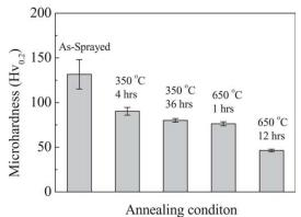
Figure 10: The effect of annealing on microhardness of the coated specimen [48].
