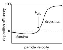
Figure 5: The effect of particle velocity on deposition efficiency in CGDS [22].
