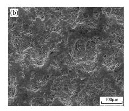
Figure 12: Surface morphology of as-sprayed NiCrAlY bond coating (a) and after shot-peened NiCrAlY bond coating (b)[58].
