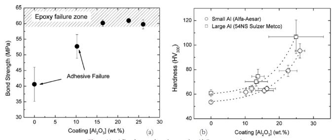
Figure 11: a) Bond strength against coating Al<sub>2</sub>O<sub>3</sub> concentration; b) Vickers hardness measurements against Al<sub>2</sub>O<sub>3</sub> concentration [52].
