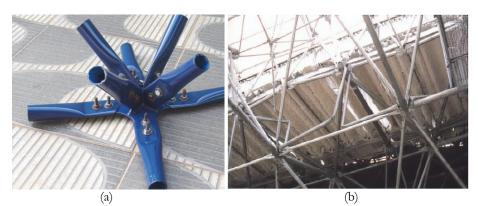
Figure 1: Connection configuration of the end-flattened steel bars (a) and the collapse of a three-dimensional truss (b) [1].
