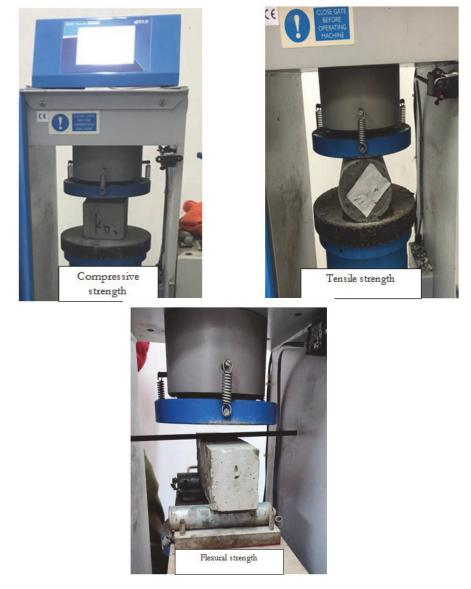
Figure 4: Hardened properties Tests.
