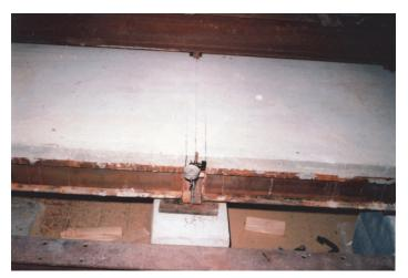
Figure 21: Dial (5) Position to Record slippage in All Models.
