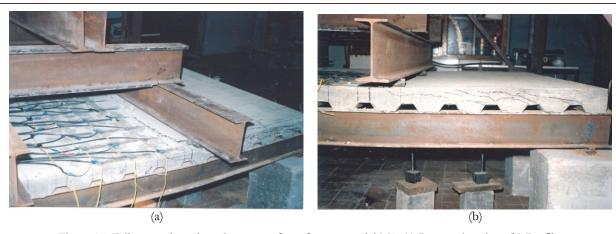
Figure 34: Failure mode and cracks pattern for reference model M1. (a) Perspective view; (b) Profile.
