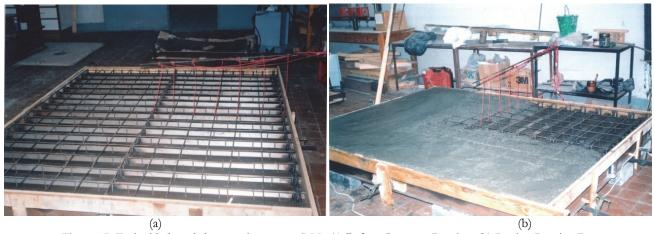
Figure 17: Embedded steel sheet strain gauges; (M1). (a) Before Concrete Pouring; (b) During Pouring Process.
