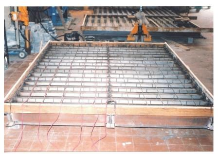
Figure 12: Reinforcing Steel Bars Top Mesh; (M1).
