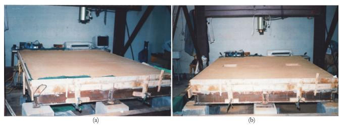
Figure 13: Final state of sand layers application (uniform distributed load). (a) Uniform load (M1); (b) Uniform load (M2).
