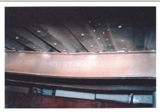
Figure 36: Typical steel beams and steel sheets yielding state for all models.
