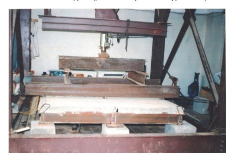
Figure 14: Loading system arrangements (concentrated loads).
