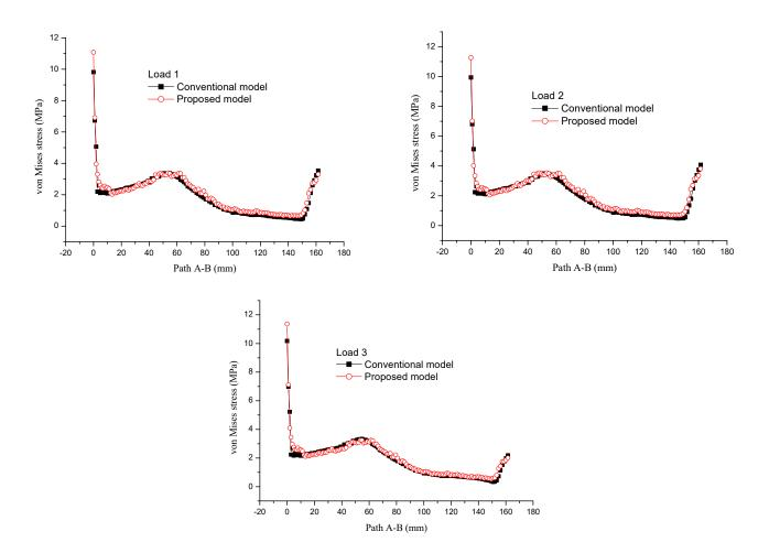
Figure 6: von Mises stress distribution along the cement path A-B for the three loading cases in the two models.
