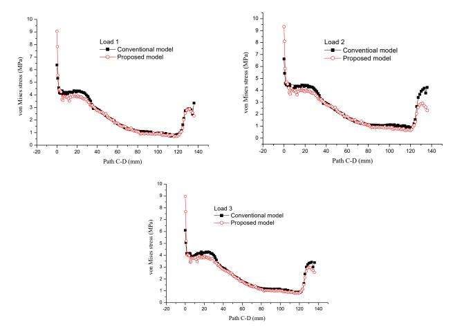
Figure 7: von Mises stress distribution along the cement path C-D for the three loading cases in the two models.
