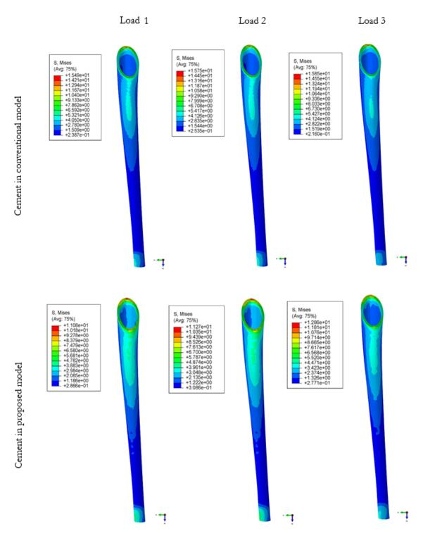
Figure 4: von Mises stress in the cement of both conventional and proposed models
