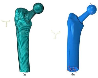
Figure 3: (a) Typical mesh, (b) Loading and boundary conditions.
