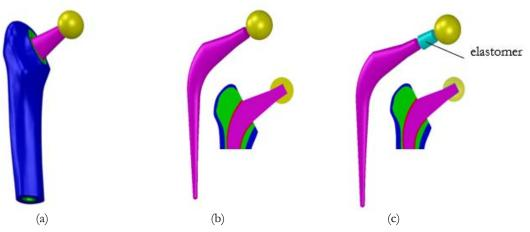
Figure 2: (a) Full model, (b) Detailed conventional model, (c) Detailed proposed model.
