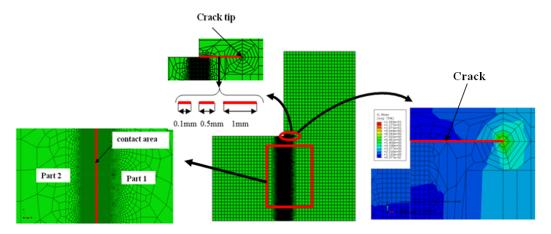
Figure 7: FEM model and contact zone in the case  $\alpha = 0^{\circ}$ .
