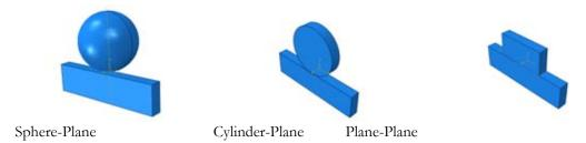
Figure 4: Different geometric configurations used for fretting tests.
