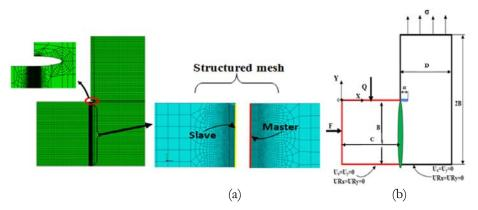
Figure 5: Model to model fretting fatigue and initial cracking; a) Slave-Master model of fretting fatigue; b) boundary conditions and dimensions of model.
