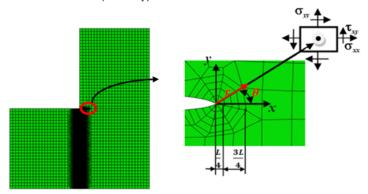
Figure 2: Stress field in the crack front vicinity
