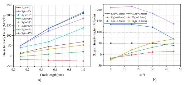
Figure 13: SIF evolution: a) as a function of the crack length (a); b) as a function of the angle ( $\alpha$ )
