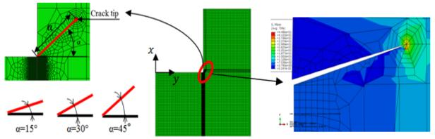
Figure 10: Fretting fatigue model with an initial inclined crack  $\alpha = 15^{\circ}$ , 30° and 45°.
