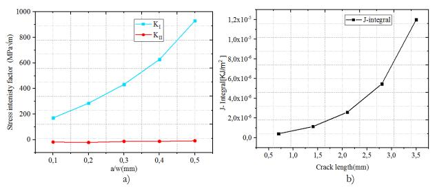
Figure 6: The variation of the SIF factor along the ratio (a/w) a); and b)The variation of the (J) in function of crack length.
