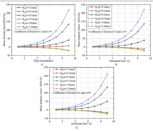
Figure 8: The evolution of the FIC as a function of time increment with COF a) 0.1, b) 0.3 and c)  $0.6\alpha = 0^{\circ}$ .
