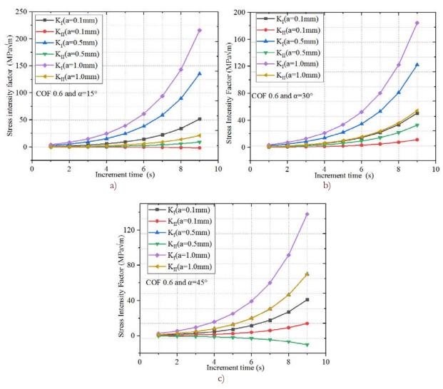
Fig. 11: The evolution of the FIC as a function of time increment with COF 0.6 and  $\alpha = 15^{\circ}$ , 30° and 45°.
