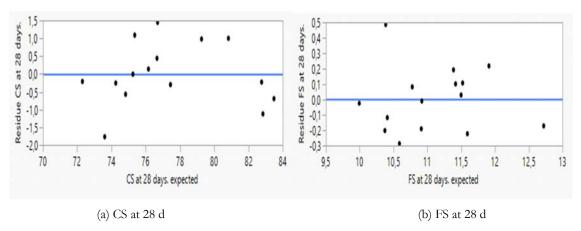
Figure 5: Graph perform the residues as a function of the predicted values at 28 days.
