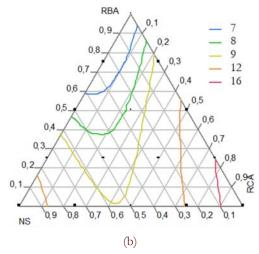
Figure 3: (a) Graphical representation of observed and predicted slump for the 15 tests, (b) Iso-response curves of slump of HPCs as function of substitution rates of the three types of sand (NS, RBA, RCA).
