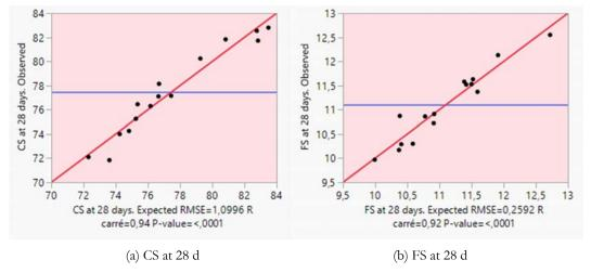
Figure 4: Graph representing the observed values as a function of the predicted values for the mechanical strength.
