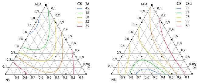
Figure 7: Iso-response curves for the compressive strength at 7 days and 28 days.
