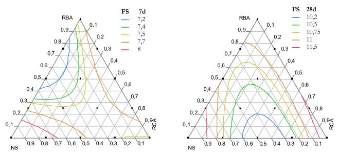
Figure 6: Iso-response curves for the flexural strength at 7 days and 28 days.
