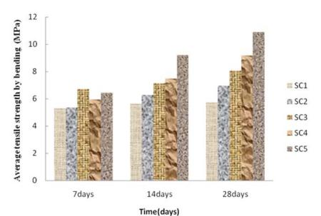
Figure 6: Tensile strength by bending of the study SC at 7 days, 14 days and 28 days.
