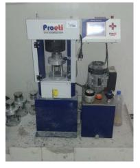
Figure 3: Machine for compresiion test.
