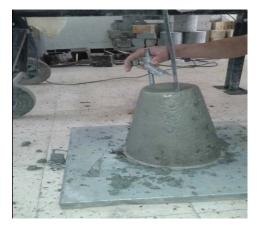
Figure 5: Sagging of plastic concrete (SC3, SC4).
