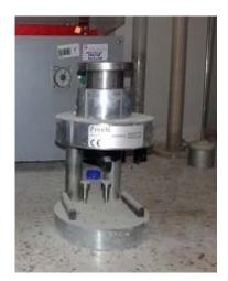
Figure 2: Tensile machine, three point bending test.
