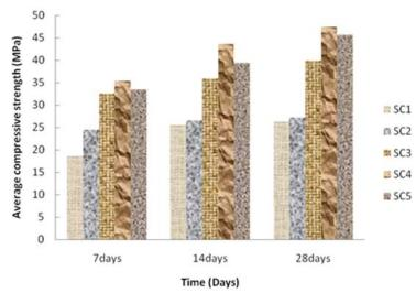
Figure 7: Compressive strength of study SC at 7 days, 14 days and 28 days.
