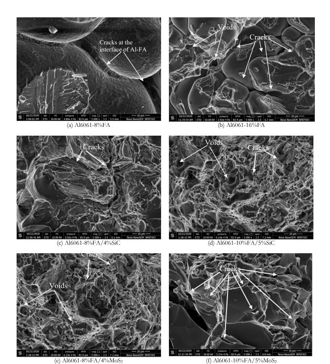
Figure 8: SEM of fractured surfaces of the aluminum hybrid composites
