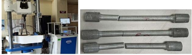
(b): Tensile testing experimental setup
