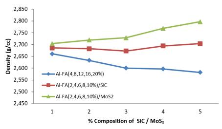
Figure 4: Density of hybrid aluminum matrix composites
