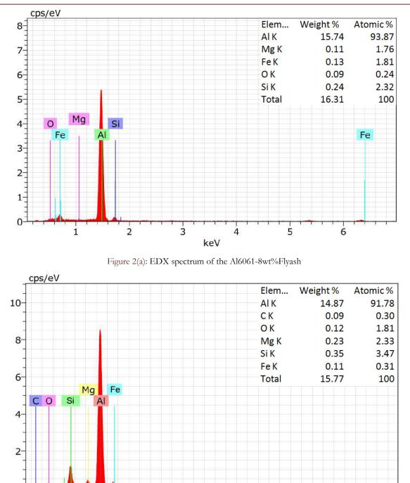
Figure 2(b): EDX spectrum of the Al6061-6wt%FA/ 3wt%SiC composite.
