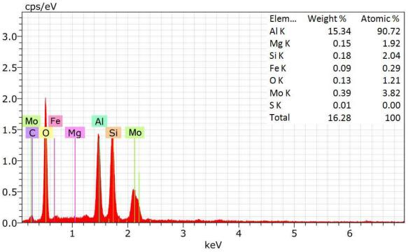
Figure 2(c): EDX spectrum of the Al6061-6wt%FA/ 3wt%MoS2 composite.
