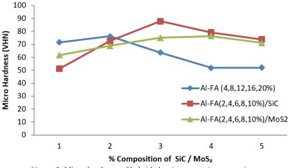
Figure 5: Micro-hardness of hybrid aluminum matrix composites
