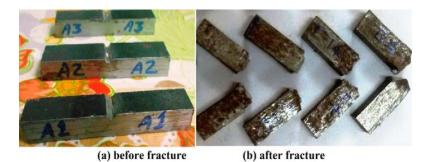
Figure 1: toughness test samples.
