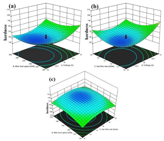
Figure 4: Response surface plot showing the interation effect of (a) WFS Vs V,(b) GFR Vs and V and (c) GFR Vs WFS on hardness.
