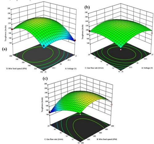
Figure 2: Response surface plot showing the interation effect of (a) WFS Vs V,(b) GFR Vs and V and (c) GFR Vs WFS on toughness.
