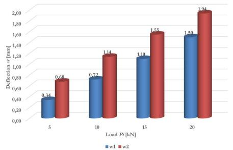
Figure 12: Results of measurements of deflection in the center of the slab, at various loads with concentrated force Pi in the geometric center of the slab, normal to its surface, where:  $w_1$  – the load was applied from the side of the titanium layer,  $w_2$  – the load was applied from the side of the steel layer.
