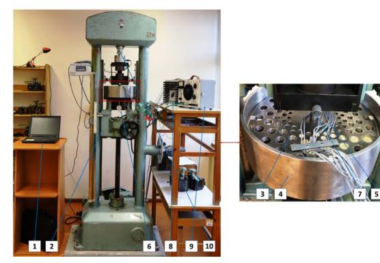
Figure 6: View of the testing machine prepared for testing in the case of plate loading with concentrated force P, where: 1 - computer, 2 - universal testing machine, 3 - steel-titanium circular axially symmetrical perforated plate, 4 - annular support, 5 - strain gauge, 6 - sensor dial, 7 - pressure pin, 8 - distribution box, 9 - strain gauge bridge, 10 - dial gauge.
