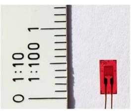
Figure 3: Strain gauges type: Tokyo Sokkia Kenkyujo Co Ltd, FLA-1-11.
