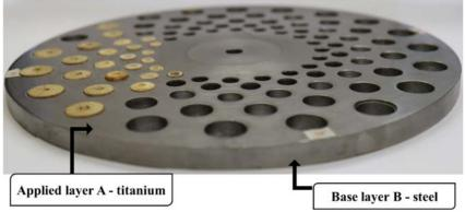
Figure 2: Model of bimetallic perforated plate.
