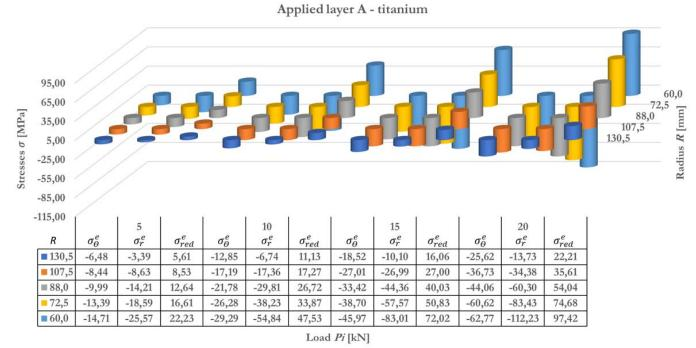
Figure 8: Summary of the stress values, respectively:  $\sigma_{\theta}$ ,  $\sigma_r \sigma_{red}$  determined on the surface of the applied layer of the plate A – titanium, in this case, the load was applied from the side of the titanium layer.
