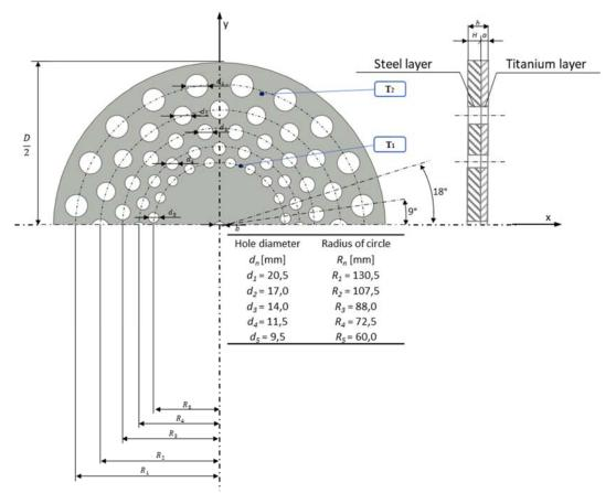
Figure 1: Model of bimetallic perforated plate consisting of steel thickness perforated plate H and titanium perforated plate thickness a containing holes with diameters  $d_1, \ldots, d_5$ .
