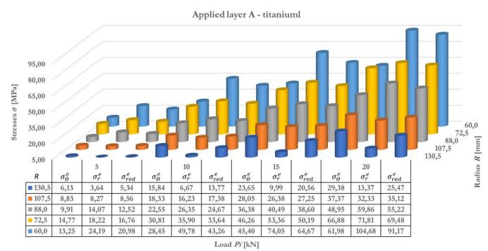
Figure 10: Summary of the stress values, respectively:  $\sigma_{\theta}$ ,  $\sigma_r \sigma_{red}$  determined on the surface of the applied layer of the plate A – titanium, in this case, the load was applied from the side of the titanium layer.
