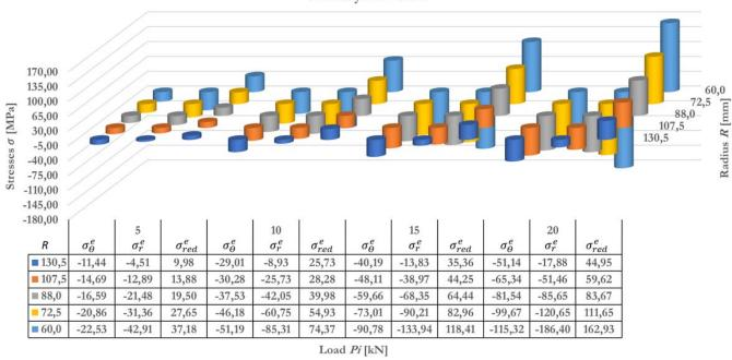
Figure 11: Summary of the stress values, respectively:  $\sigma_{\theta}$ ,  $\sigma_r$ ,  $\sigma_{red}$  determined on the surface of the base layer of the plate B – steel, in this case, the load was applied from the side of the steel layer.
