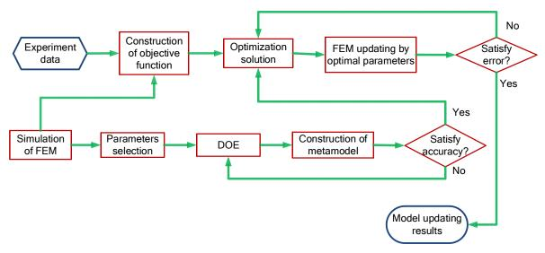
Figure 6: Flow chart of the process of model updating.
